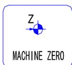
**Machine zero return in Z direction:** It is valid in “Jog”/ “Auto” mode. (whether machine zero return is valid is defined by MZRO bit of P12)
