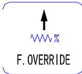
**Increasing feedrate override:** Increase feedrate override in “Jog” mode and G01 feedrate override in “Auto” mode.
