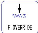
**Reducing feedrate override:** Reduce feedrate in “Jog” mode and G01 feedrate override in “Auto” mode.
