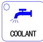
to switch the coolant ON/OFF. Start the coolant, and the system displays the coolant is **ON** and LED is **ON**; stop the coolant, and the system displays the coolant **OFF** and LED **OFF**.
