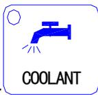
is pressed, the coolant ON/OFF is switched. When the coolant is ON, LED is ON, the corresponding bit of M8 in output 1 is 1 and that of M9 is 0; when the coolant is OFF, LED is OFF, the corresponding bit of M8 in output 1 is 0 and one of M9 is 1.
