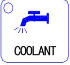
Coolant ON/OFF: After starting the coolant, the system displays **COOLANT ON** and LED is ON; after stopping the coolant, the system displays **COOLANT OFF** and LED is OFF.
