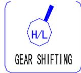
to change the spindle speed. If it is pressed once, the spindle speed is output circularly S1, S2, S3, S4,(SCOD=0) or S0~S15 (SCOD=1). The spindle
